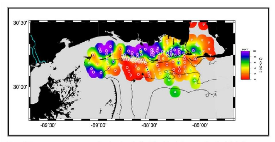
Figure 1. Bottom-water oxygen concentrations (ppm), recalculated from historical core-top data. Symbols indicate published source of core-top data. Circles are from Phleger (1954), triangles from Parker (1954), and inverted triangles from Puckett (1992), as described by Brunner et al. (2006).
