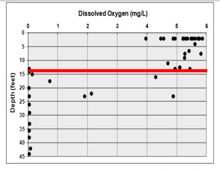
Figure 6: Graph showing dissolved oxygen with depth in 2011. Notice a decline of dissolved oxygen with depth and the rapid decline in oxygen around 10-20 feet deep.
