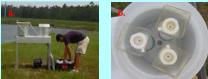
Figure 2a. Aerochem sampler at the Pace sampling site showing the in field setup and b. the bottle and funnel setup.
