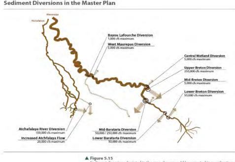
Sediment diversions depicted in the map above would be operated in coordination with high river events and seasonal flows. Operation at maximum capacity would occur only at targeted intervals for a fraction of time each year.
