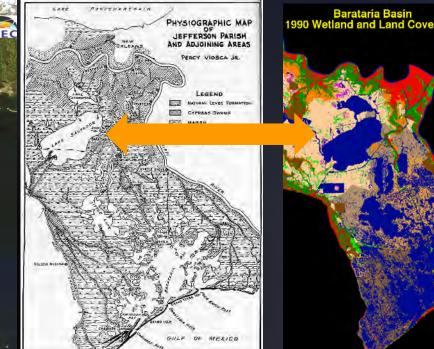
River abandonment caused by levees along the Mississippi River, reducing sediment delivery to wetlands (see sediment plumes in satellite image), has caused a shift from prograding to transgressive processes to dominate along the deltaic coast.
