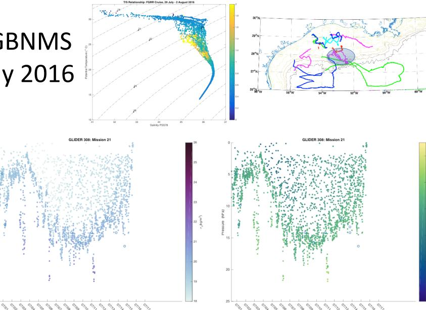
Despite being in water depths > 100 m, the glider was unable to penetrate the pycnocline at 10-15 m.
