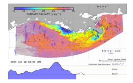
Visualization of hydrodynamic model showing sea surface salinity in relationship to Mississippi River discharge in 2009. Source: S. DiMarco, Texas A&M
