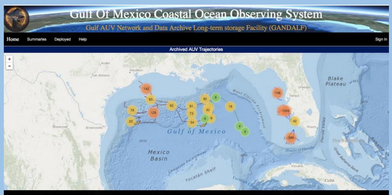
The GCOOS-RA developed the Gulf AUV Network and Data Archive Long-term storage Facility (GANDALF) to provide data management and glider mapping/tracking assistance to glider operators in the Gulf.
