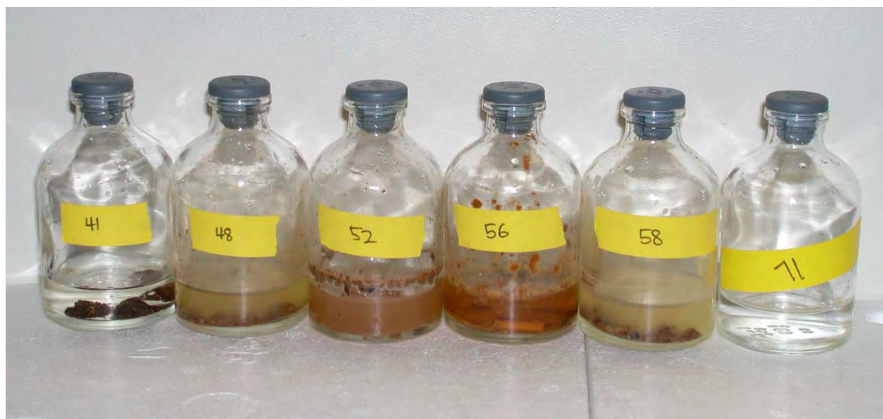
Figure 2. Photograph of a sample from each treatment at day 50. Treatments are from left to right: Seawater +tarballs (41); Seawater+tarball+N+P (48); Seawater+tarball+N+P+Molassas (52); Seawater+tarball+N+P+Switchgrass (56); Seawater+tarball+N+P+Naph+Hex (58); Seawater only (71)
