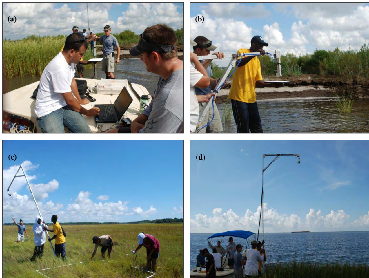
Fig 2a – 2d: Field Survey, (a) Ocean Optics Setup, (b) Calibration using 99% panel, (c) Acquiring LAI and Chlorophyll readings, (d) Reflectance Measurement.
