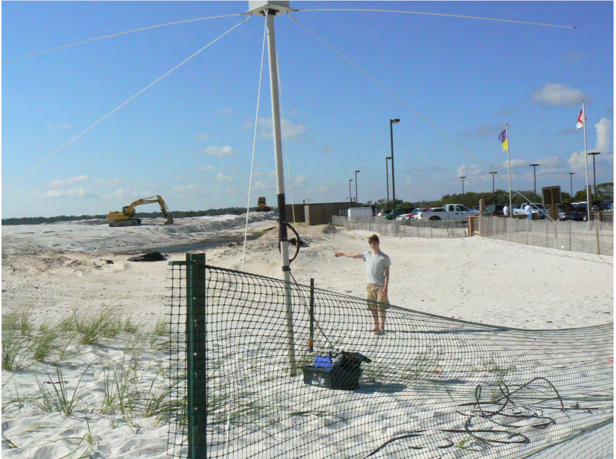
Figure 4. CODAR receive antenna at Orange Beach, AL, shortly after reinstallation at Gulf State Park. Work on the ongoing dune replenishment project is seen in the background to the left. The white utility trailer in the background houses the CODAR electronics .
