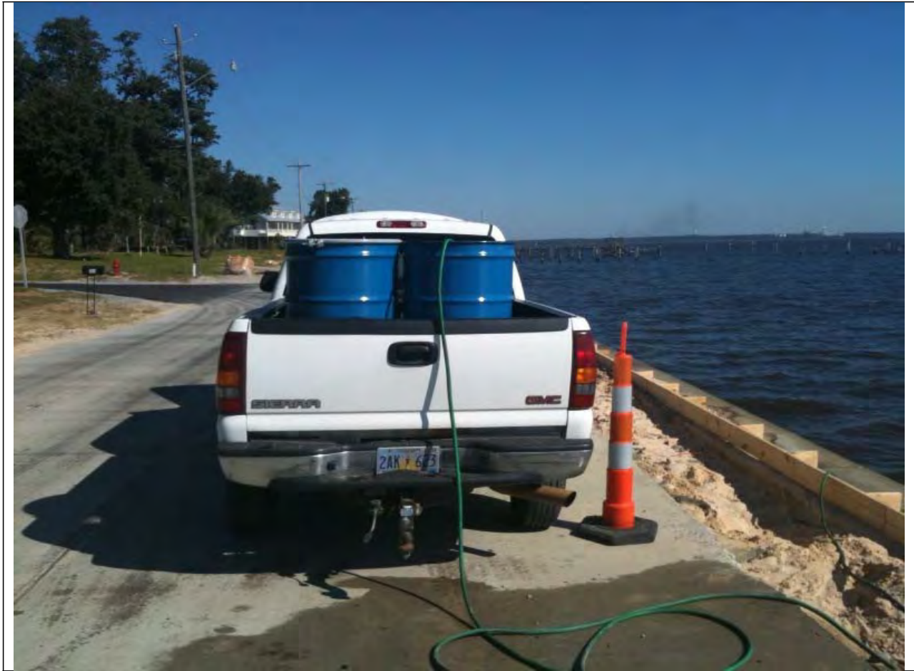
Figure E3B.2 Apparatus to collect water samples
