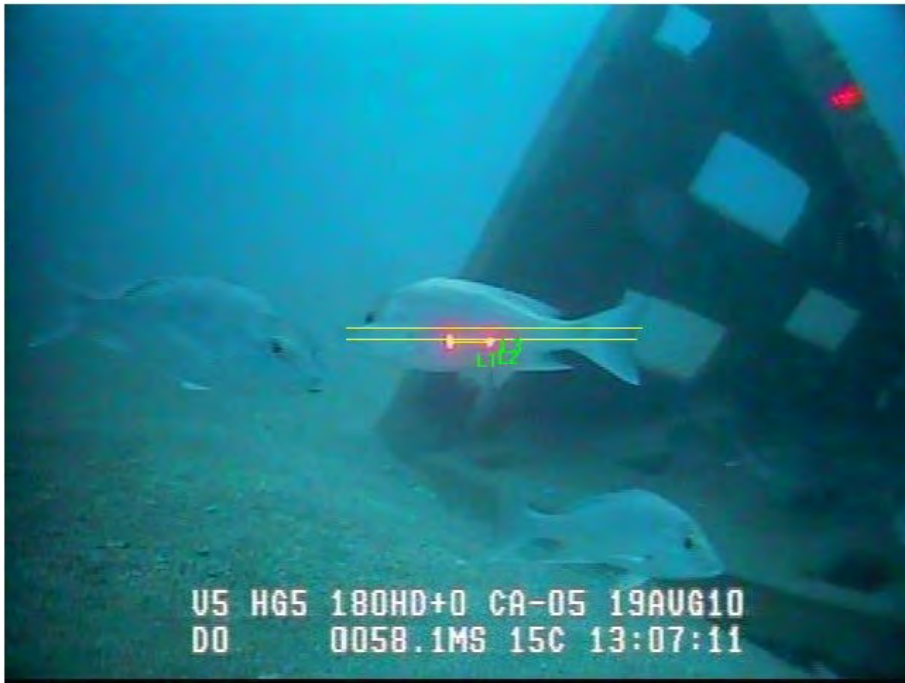
Example of footage from the ROV taken on August 19, 2010 showing the laser-based method of obtaining length data. Image credit Dauphin Island Sea Lab.
