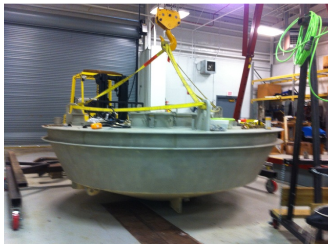
Figure 13. Sandblasted hull of 3-m discus buoy modified by the National Data Buoy Center to house the PMEL MAPCO 2 system
