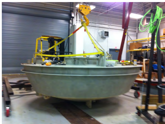
Figure 5. Sandblasted hull of 3-m discus buoy modified by the National Data Buoy Center to house the PMEL MAPCO 2 system
