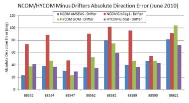
Figure 1 .Example of validation for eight drifter-derived ocean current speed and direction in 2010 June.
