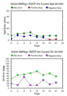
at 2 m. The x axis represents the analysis time, 3-, 6-, 9-, 12-, 15-, 18-, and 21-h forecast. The y axis represented direction error and speed error. One line represents absolute error, and is shaded green. Another line represents bias; speed bias is shaded blue for negative values and red for positive values, while direction is shaded purple for negative values and magenta for positive values (Fig. 23).
