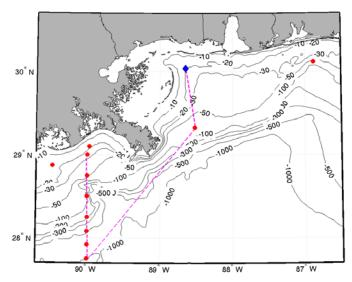
Figure 5. Wave Glider trasects. The magenta line is the 242 km waveglider track. Assuming a speed of 0.6 knots, the round-trip transit time is 18 days. GOMEC2 stations are red circles and the CenGOOS buoy is a blue diamond.
