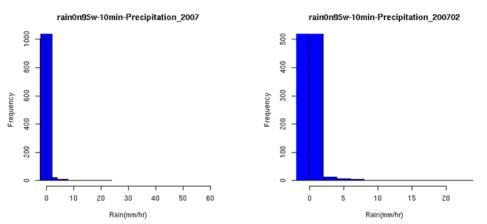
Figure 10. Example of histogram plots for rain rate (mm h-1) in ten-minute intervals for the buoy located on the equator at 95°W. An instance of annual data distribution in 2007 is shown on the left, and February 2007 shown on the right. Note the contaminated negative values.
