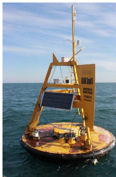
Figure 17 Buoy USM3m01 photo taken on December 11, 2015. One of the two anemometer masts and the antenna mast are gone. One of the NOAA/NDBC modules used for testing new components for their SCOOP system is seen dangling in the water. Although one anemometer mast remains, the anemometer is missing.
