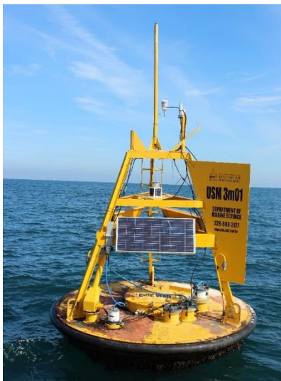
Figure 19 Buoy USM3m01 with operational MAPCO2 system. The Iridium antenna is the cone shaped antenna on the smaller mast stub to the right side.
