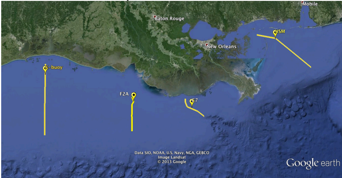
Figure 7. Proposed repeat glider transects. Each of these transects runs from the 10 m to the 60 m isobath. Mooring USM is operational, but it requires a bottom package for seafloor dO. Real-time mooring stations at F2A, C6 and along the K-line are proposed.
