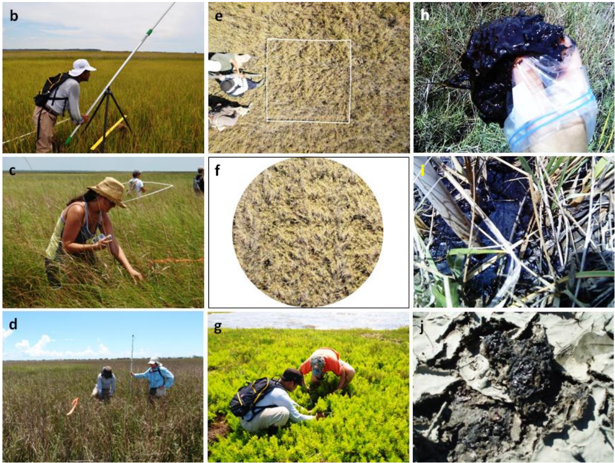
Figure 6: Top of Canopy reflectance measurement using OceanOptics USB4000 spectroradiometer, c: Measurement of leaf level chlorophyll using Konica-Minolta SPAD 502 chlorophyll meter, d: Leaf Area Index (LAI) measurement using AccuPAR LP-80 Ceptometer, e & f: Vegetation Fraction measurement using vertical digital photograph, g: Above ground biomass collection from a 1 sq. ft plot within the IFOV of the sensor, h, i and j: Residual oil and dispersant observed in survey locations.
