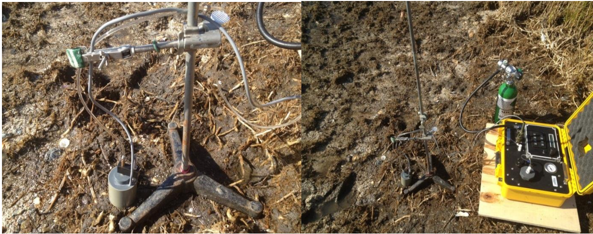
Image 3: CSM sensor head close view (left) and the entire CSM setup (right).
