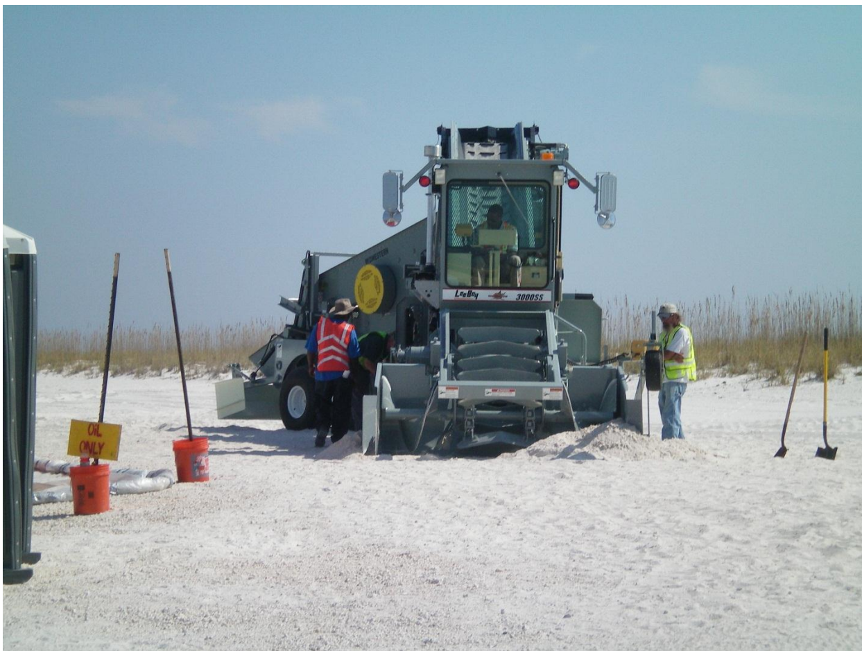
Fig. 1. Machine for beach deep cleaning at Pensacola Beach (Photo: Huettel)
