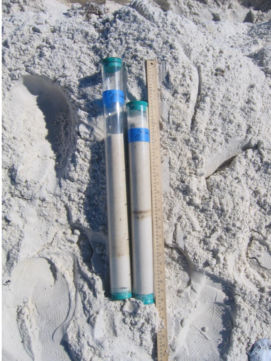
Fig. 6 Sediment cores retrieved after the deep cleaning process showing layer of dispersed oil particles. (Photo: Huettel)
