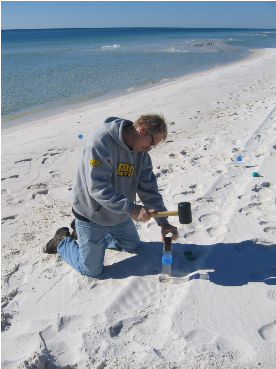
Fig. 5 Sediment coring at Pensacola Beach (Photo: Huettel)
