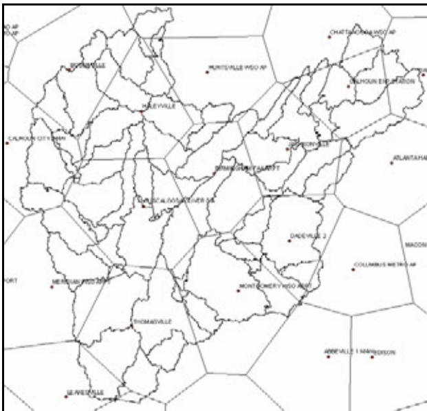
Figure 7. Meteorological stations and Thiesen polygons for assigning meteorological data to sub-basins. Weather stations were changed during the calibration process by comparing rainfall patterns with measured hydrographs. This comparison helped in deciding what weather station was more representative for a particular sub-basin (hence, the initial weather station assignment done according to Thiesen polygons was modified during calibration).
