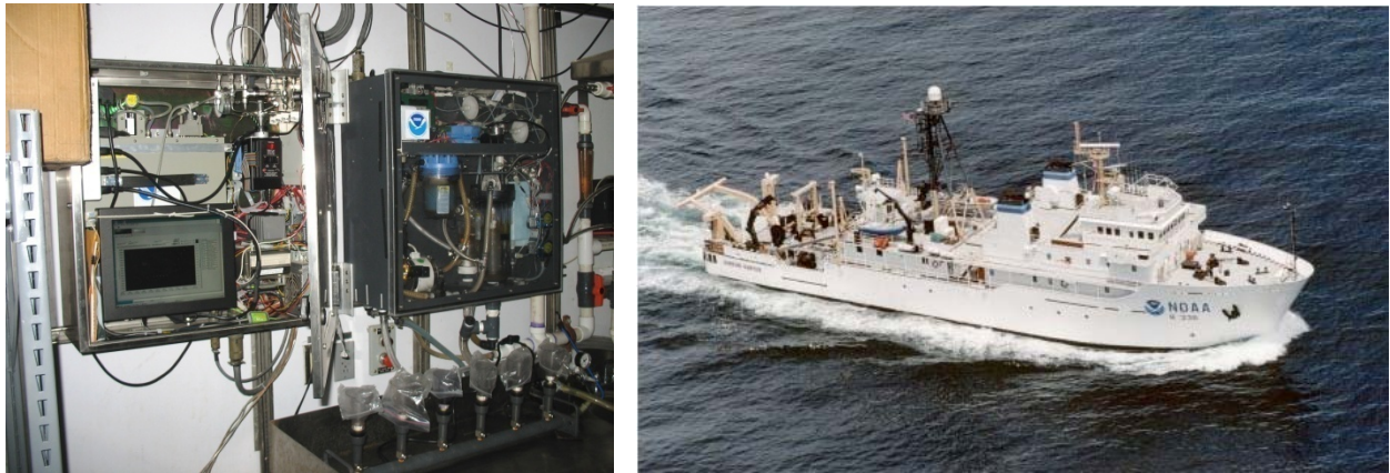
Figure 32. Installation of the autonomous pCO 2 system (left) on the NOAA ship Gordon Gunter (right) occurred in March 2008.
