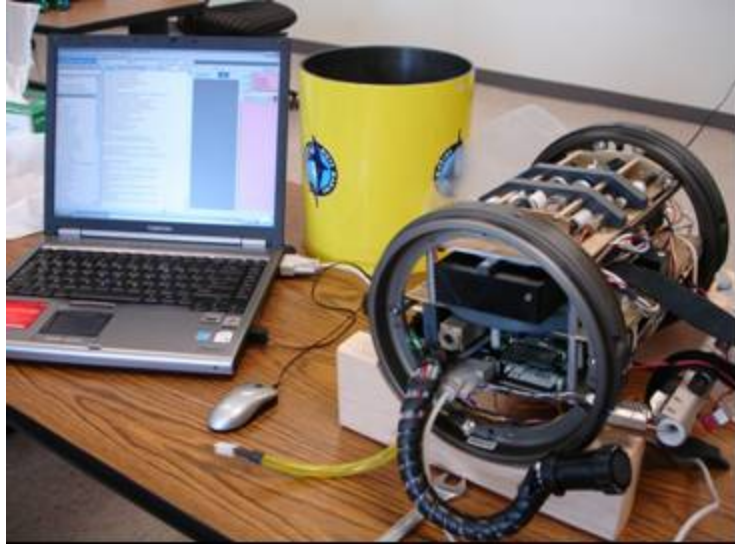
Figure 76. Optical Plankton Discriminator designed as a payload for a Web Slocum glider.
