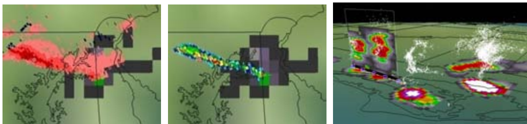
Figure 46. Rotation track, hail swath, and IC lightning data for a tornadic storm on 17 July 2007, and a cross-section of total lightning sources and source density.
