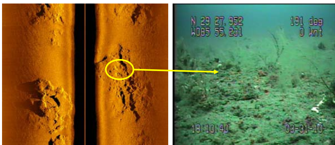
Figure 65. Side scan image and geo-referenced drop camera image of low relief rocky habitat in the Three-by-fives.
