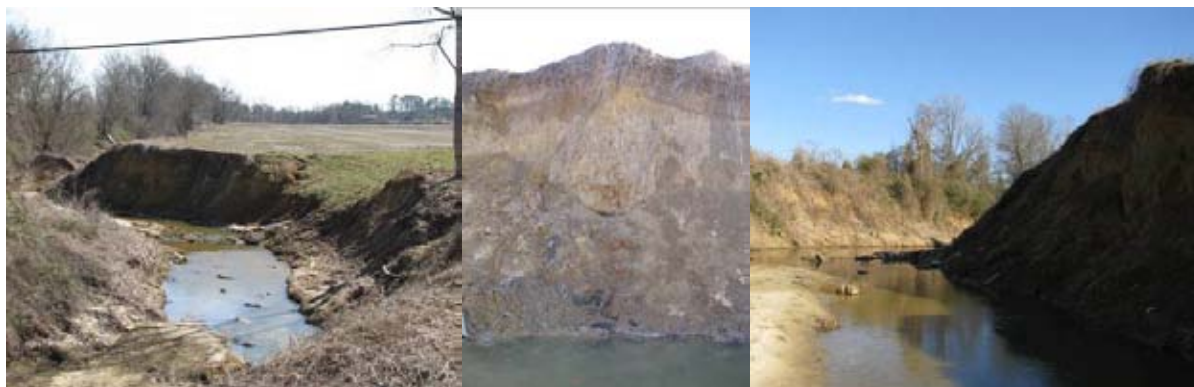
Figure 23. Surveyed cross sections to determine streambank erosion and bank instability at Yonaba Creek, MS
