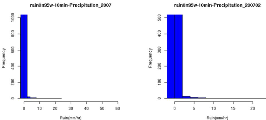
Figure 10. Example of histogram plots for rain rate (mm h<sup>-1</sup>) in ten-minute intervals for the buoy located on the equator at 95°W. An instance of annual data distribution in 2007 is shown on the left, and February 2007 shown on the right. Note the contaminated negative values.
