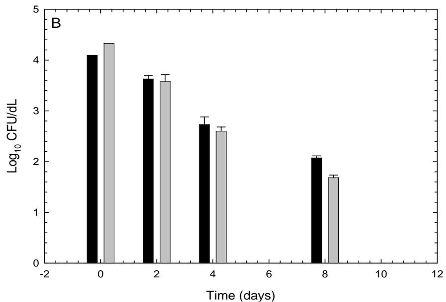
Figure 26. Survival of sewage enterococci in October 2012 at a public beach in Pass Christian. Black bars are filtered beach water and sewage and grey bars are natural beach water and sewage. Error bars are standard errors of four replicates.
