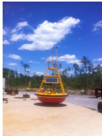
Figure 33. Buoy running a burn-in test at the USM Oceanographic Support Facility at Stennis Space Center, MS
