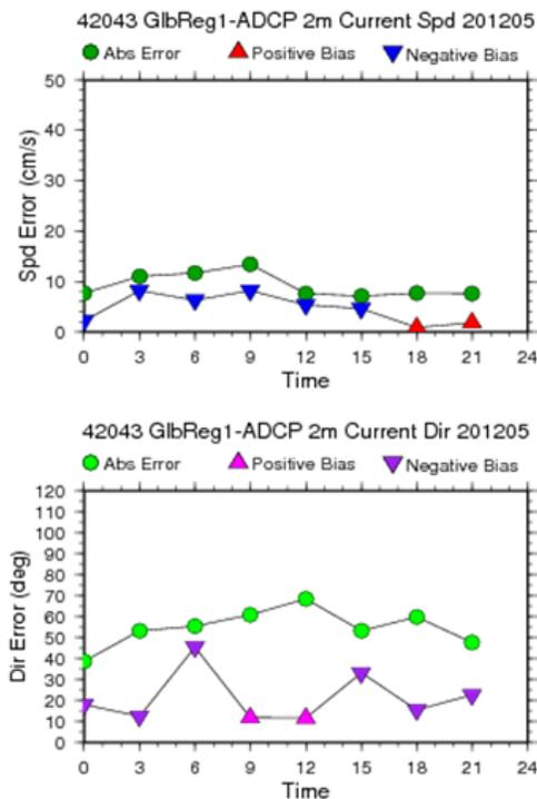
at 2 m. The x axis represents the analysis time, 3-, 6-, 9-, 12-, 15-, 18-, and 21-h forecast. The y axis represented direction error and speed error. One line represents absolute error, and is shaded green. Another line represents bias; speed bias is shaded blue for negative values and red for positive values, while direction is shaded purple for negative values and magenta for positive values (Fig. 23).
