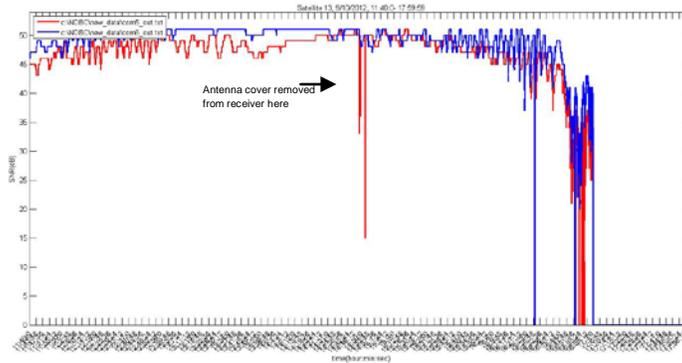
Figure 6. Example of results from the analysis of antenna-received data between a PVC-covered and uncovered AERO antenna. Very minimal dB differences existed between the two. The differences were less than 2 dB even with the sandwich radome. This difference should not present any problems in the analysis of data.
