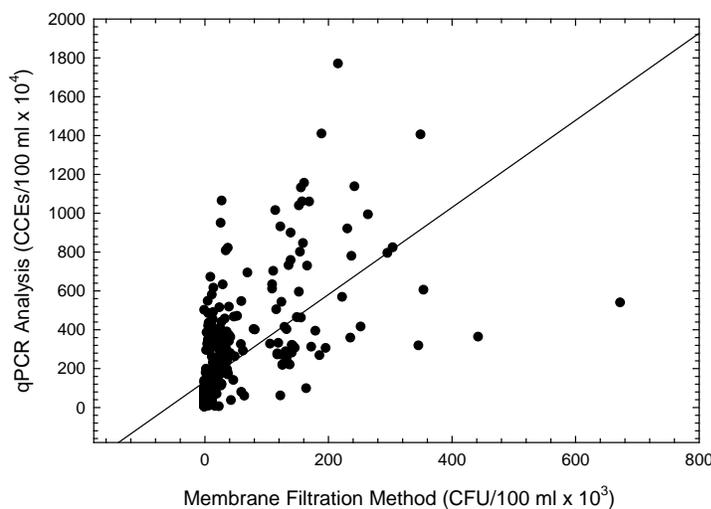
Figure 28. Regression analysis comparing results obtained using two methods of determining enterococci concentration in water. One is a culture-based using membrane filtration and the other is molecular-based using qPCR.  $Y = 2.2411X + 133.7$ ;  $r^2 = 0.3881$
