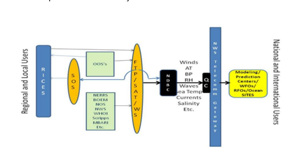
Figure 36. The functional diagram of NDBC’s data aggregation and dissemination architecture.
