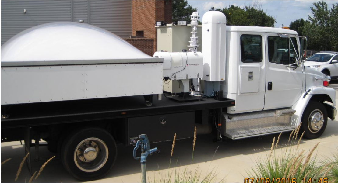
Figure 74 RaDAPS instruments, from left to right: DeTect 915 MHz wind profiler antenna, Radiometrics microwave profiling radiometer, surface instrument cluster on a telescoping tower (in folded position behind the radiometer), and a Vaisala CL-51 LIDAR ceilometer. A Mesodome™ 360° camera ( http://www.mesodome.com/ , not shown) will be mounted on top of the tan-colored computer cabinet adjacent to the telescoping tower.
