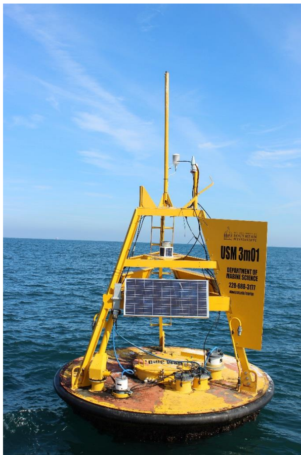
Figure 13 Buoy USM3m01 photo taken on December 11, 2015. One of the two anemometer masts and the antenna mast are gone. One of the NOAA/NDBC modules used for testing new components for their SCOOP system is seen dangling in the water. Although one anemometer mast remains, the anemometer is missing.
