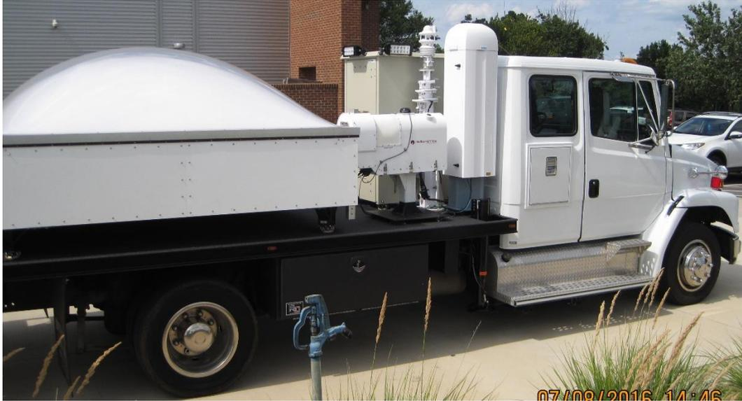
Figure 2. RaDAPS instruments, from left to right: 915 MHz wind profiler antenna, Radiometrics microwave profiling radiometer, surface instrument cluster on a telescoping tower (in folded position), and a Vaisala CL 51 ceilometer. A Mesodome 360° camera (<http://www.mesodome.com/>, not shown) will be mounted on top of the computer cabinet adjacent to the telescoping tower.
