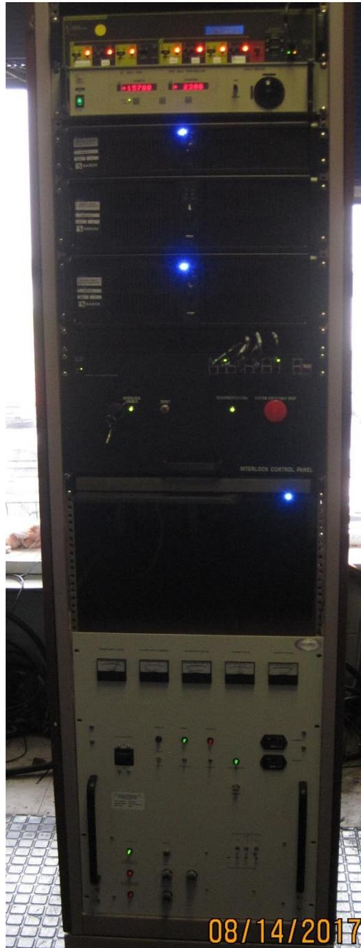
Fig. 2. ARMOR receiver components (black) are located at the top of the rack. The pre-existing transmitter assembly units are located at the bottom (cream colored).
