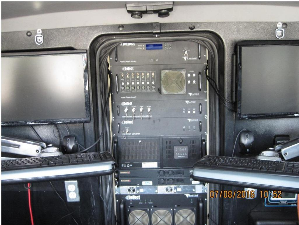
Figure 1. View of the RaDAPS computer rack and work area, located in the rear of the cab.
